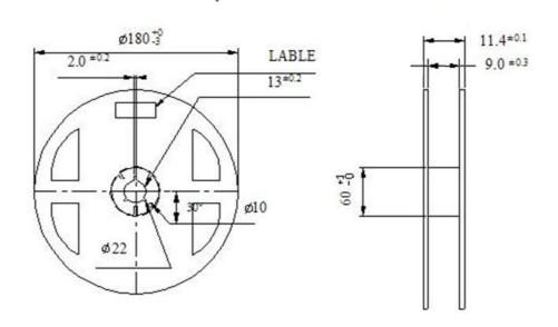
( Tolerance:  $\pm 0.2$ , Unit: mm )
