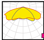
CAT Catenary street light beam optimized for EN13201 M-classes
