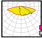
LW1 For EN13201 M-class requirements where road width > the pole height
