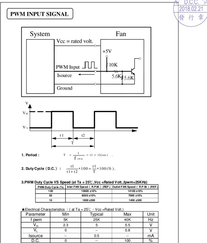
\* The speed is default to be maximum if PWM input pin is unconnected.
