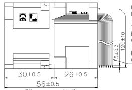
UL1571 #28AWG IN FAN +:RED(紅),-:BLACK(黑) YELLOW(黃):3rd Wire BLUE(鮭):PWM Input OUT FAN +:ORANGE(橘),-:GRAY(灰) BROWN(棕):3rd Wire GREEN(綠):PWM Input
